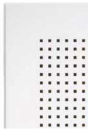
Micro, 3 x 3 mm, 8.3 mm c/c Perforation: 9.5-10.7%
